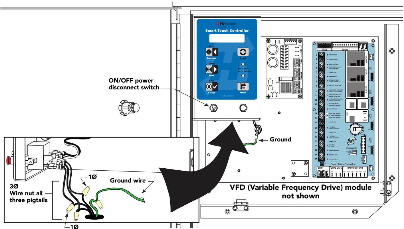
**CAUTION** \* Variable Frequency (VF) operators: Make sure the connection wires match the voltage found on the operator's nameplate.
