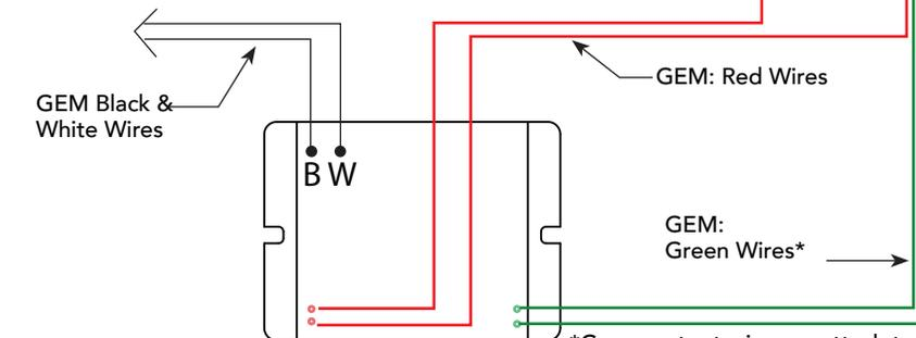
\*Green output wire can attach to any SENSOR input.
