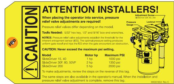
**NOTICE:** Pressure relief valve adjustments establish the threshold for the inherent entrapment sensor (IES). The optimal pressure setting produces uniform gate travel and trips the IES when the gate encounters an obstruction.
