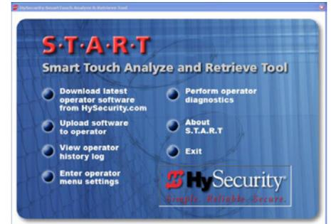
With S.T.A.R.T. software loaded on your laptop computer, you have an invaluable management tool for all HySecurity operators. The RS-232 serial port (found on the Smart Touch Controller), allows you to download system diagnostics and upload system configurations using the S.T.A.R.T. software. Instructions for downloading S.T.A.R.T. are on the website.
