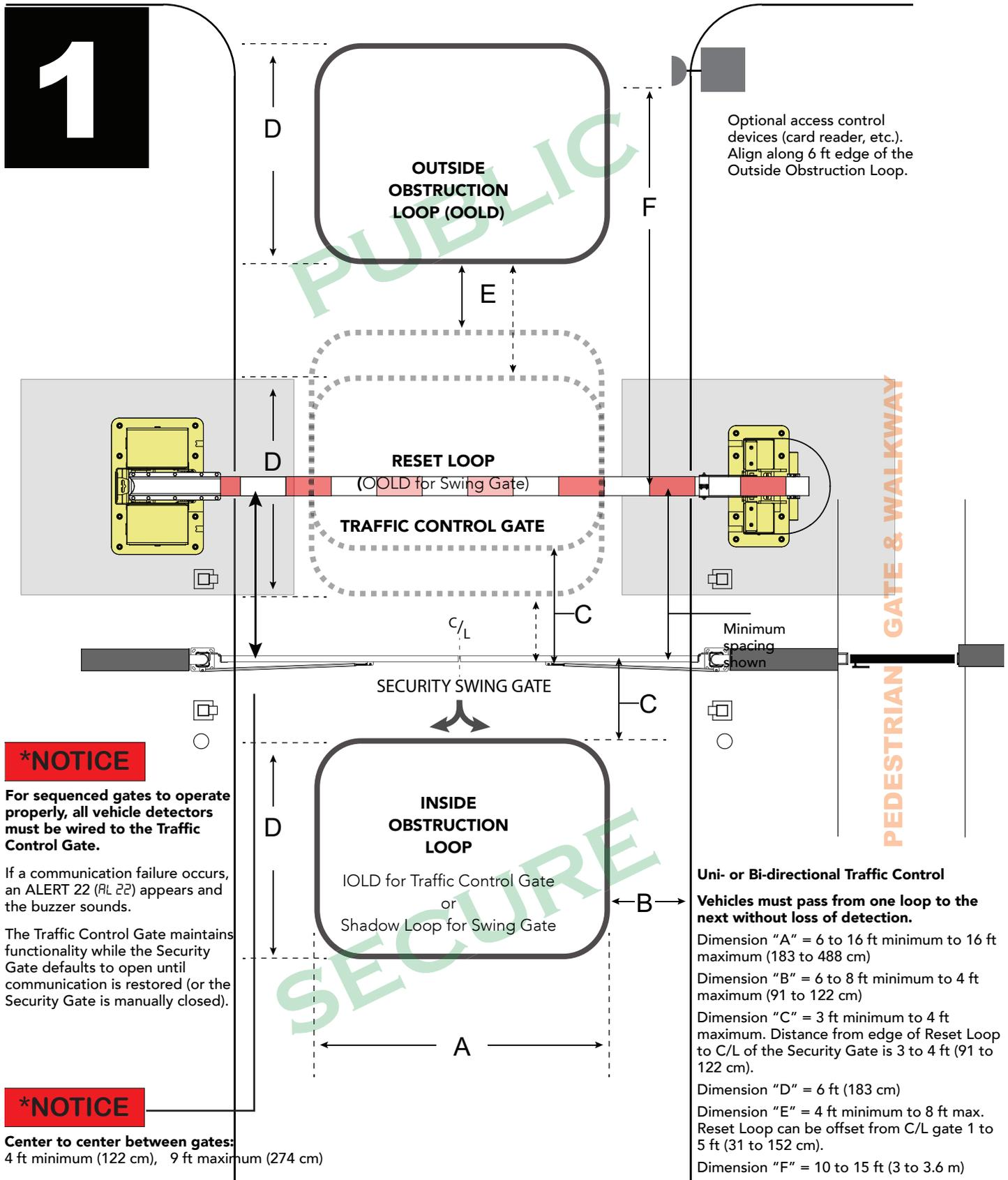
Optional access control devices (card reader, etc.). Align along 6 ft edge of the Outside Obstruction Loop.
