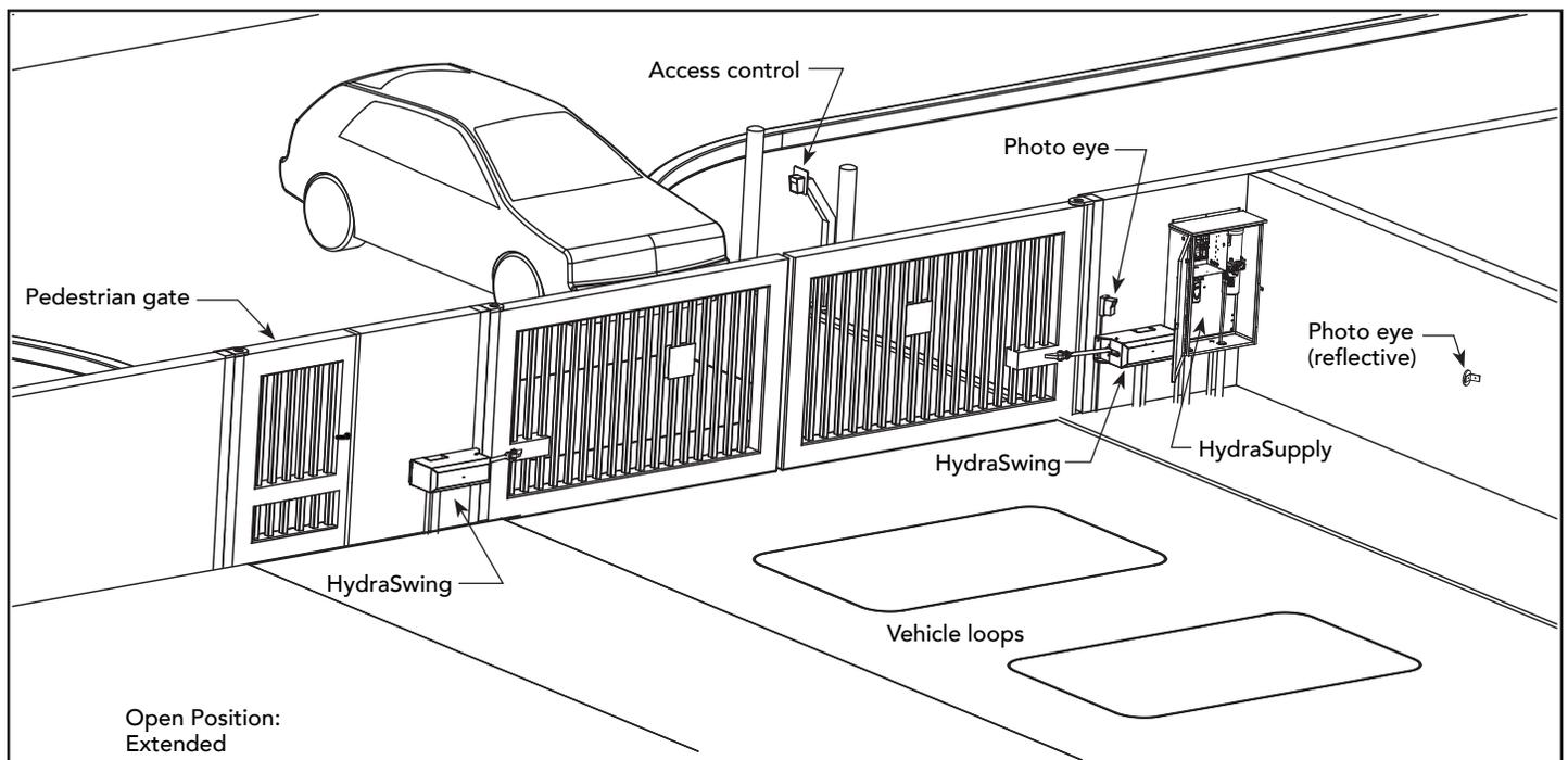
**NOTE:** To enable fully automatic operation, this gate operator requires a MINIMUM of one external entrapment protection sensor to monitor potential entrapment zones in either the open or close direction of travel.
