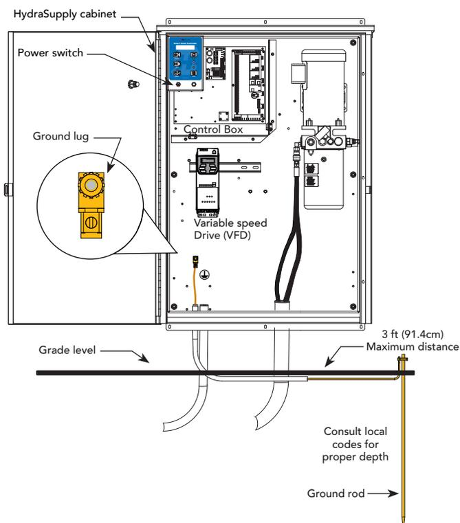
**NOTICE:** Properly grounding the gate operator is critical to gate operator performance and the life of its electrical components. Use sufficient wire size during installation. If you do not ground the operator with a separate earth ground, you risk voiding the HySecurity Warranty.
