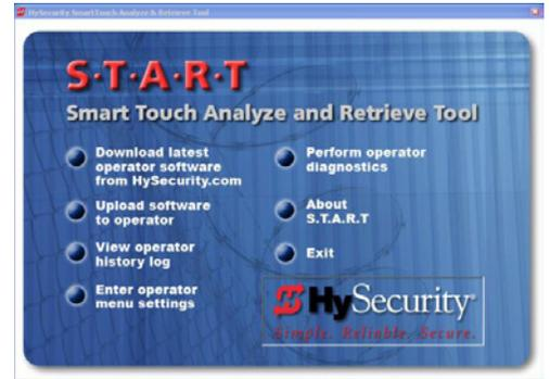
**NOTE:** Hy5A emulation mode does not include all the features of Hy5B. If you are replacing Hy5A detectors and updating the gate operator software, be aware Build Year 1 (BY1) or Build Year 2 (BY2) will need to be addressed. BY2 requires monitoring of external entrapment protection sensors per UL 325 - 2016 Standard of Safety. If the gate operator was installed prior to 2016, BY1 may be used. For more information, refer to the gate operator's product manual.
