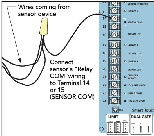
**Wire nut and pigtail to SENSOR COM**
