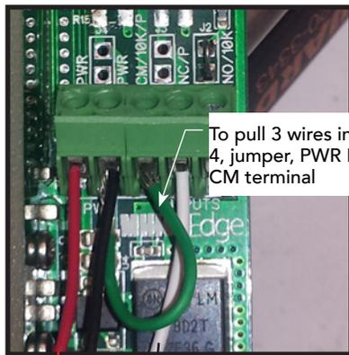
To pull 3 wires instead of 4, jumper, PWR Relay to CM terminal
