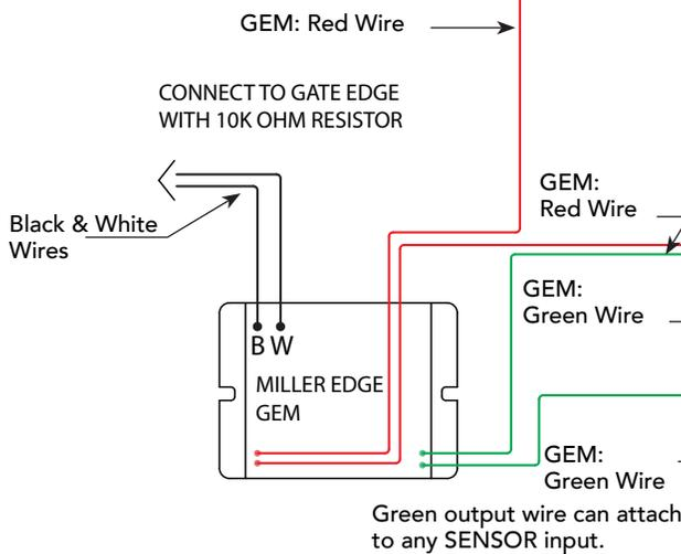
**\*NOTE:** Make sure whichever wired input used (SENSOR 1, 2, or 3) is the same Sensor # configured through the Installer Menu.
