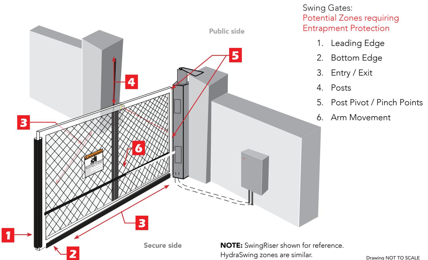
Assess your gate site for the most appropriate placement of edge sensors. Plan to integrate contact (gate edge) and non-contact (photo eyes) sensors in your site plan. Sensors are wired to the Controller and require low voltage conduit to the operator and power supply. Refer to *External Entrapment Protection Sensors monitored by HySecurity Gate Operators* on page iii.
