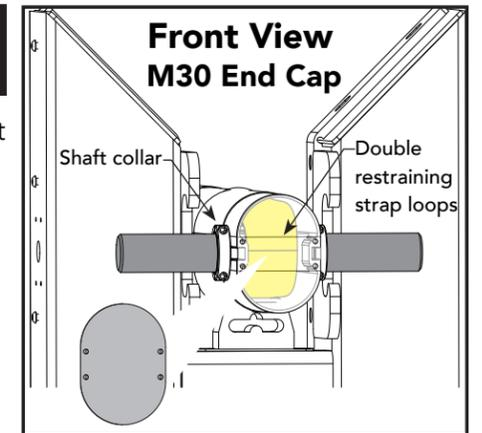
Adjust the Shaft Collars to hold the pin in place and tighten the set screws securely.
