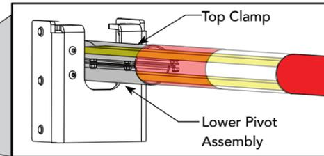
**4** Slide the Lower Arm to obtain 3/4-inch clearance at the Catch Post.
