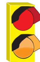
Arm lights flash when opening and closing. Default setting: **User Menu: AL 1** Arm Lights flash whenever the Close Limit is encountered. Changing to AL 0 causes arm lights to be continuously lit when the Close Limit is encountered.
