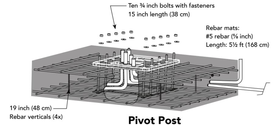
Anchor cages include 10 anchor bolts, washers, and nuts. Foundation dimensions shown: Minimum 6 x 6 x 2 ft (183 x 183 x 61 cm)
