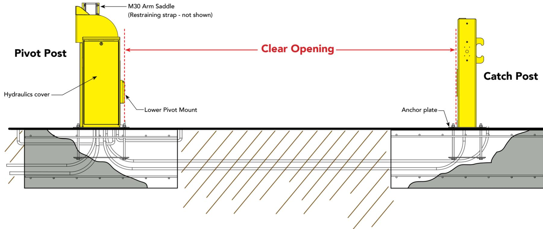
**3** Ensure the posts are plumb. Shim or grout as required.
