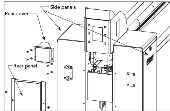
Remove the side panels, rear panel and end cap.
