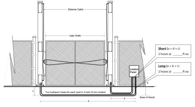
Hose, ¾", fully charged with hydraulic oil Hose fittings kit, HydraLift
