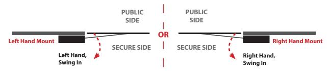
NOTE: HySecurity only provides bracket for swing-in gates, customer must fabricate their own bracket for swing-out gates.
