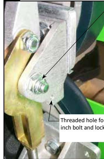
Remove the lock nut, but leave the pivot bolt in place.
