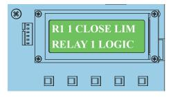
An example of a user relay function is shown here. Setting R1 to 1 creates an interlock signal to another operator's interlock input. The relay is released when the fully-closed limit switch is tripped (indicates that the gate is secure). Any open command energizes the relay.
