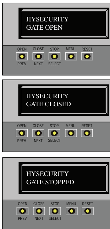
Figure 33. Gate Status Display
