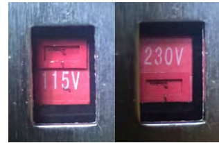
Figure 19. Voltage Switch Positions
